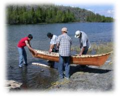
Checking for leaks
