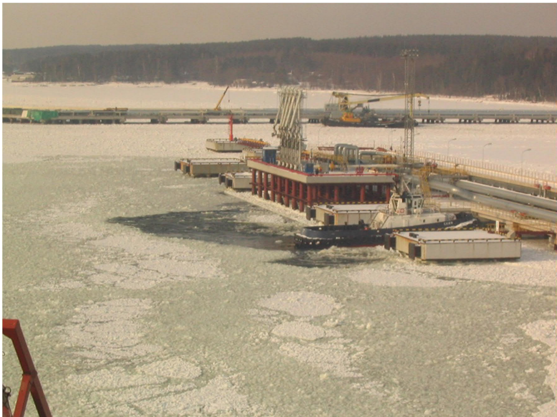
Figure 6-11 – Harbour tug is clearing the dolphins of ice by flushing with her azimuth thrusters, Eastern Gulf of Finland (Source: Aker Arctic).
