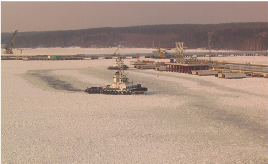
Figure 6-9 – Breaking ice before carrier arrival in the Eastern Gulf of Finland (Source: Aker Arctic)
