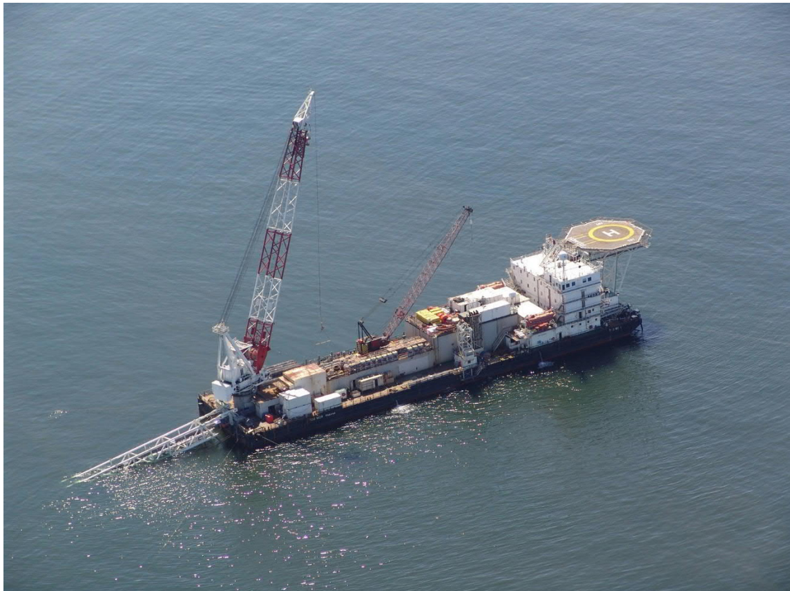
Figure 12: Typical S-Lay Laybarge
