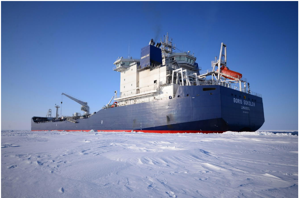
Figure 4-4 – Arctic condensate tanker Boris Sokolov during delivery ice trials in 2019 (Source: Aker Arctic)
