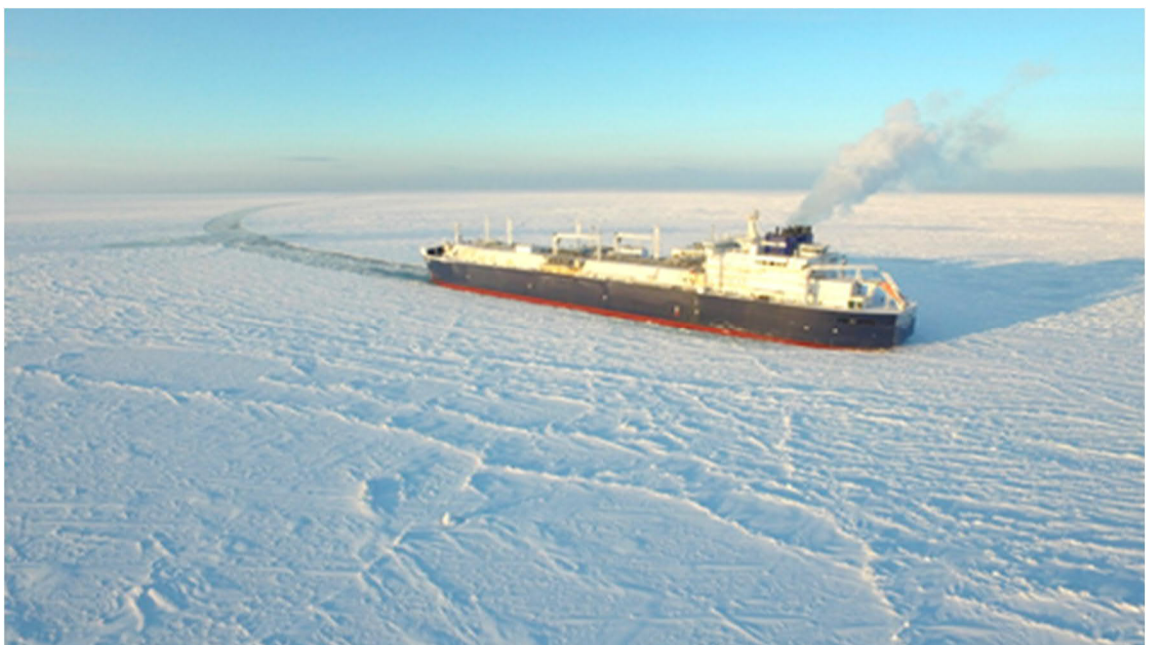
Figure 4-2 – YamalMax type LNG carrier Christophe De Margerie during delivery ice trials in 2017 (Source: Aker Arctic)
